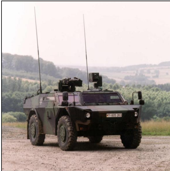
Figure 1: Military vehicle Fennek (weight 10.8 tons)
